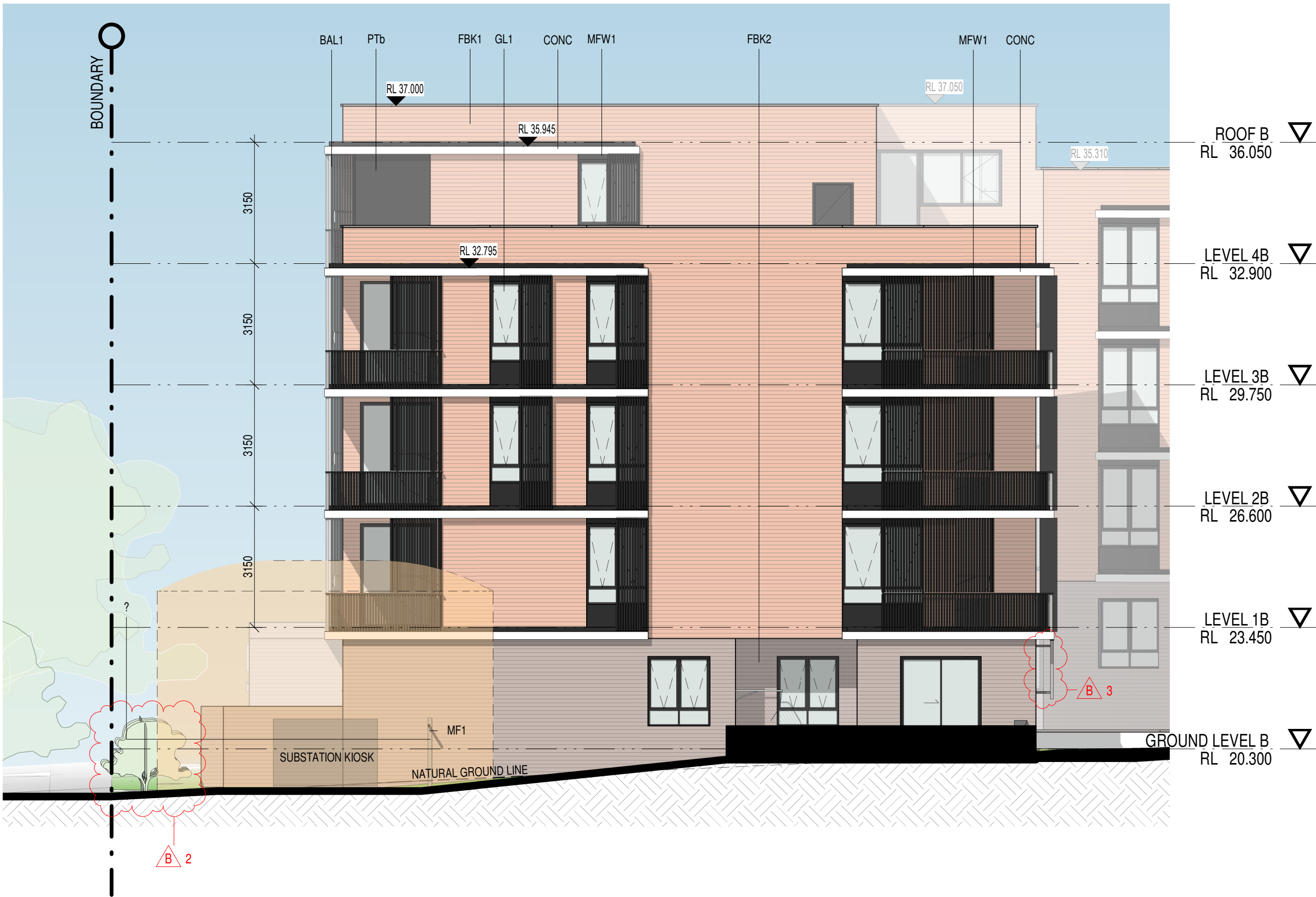
W1 DA ELEVATION - WEST (NORTHERN BUILDING) 1:100
